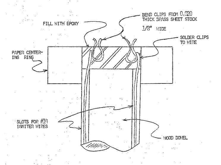
PISTON TOWER IGNITOR LEAD DETAILS
