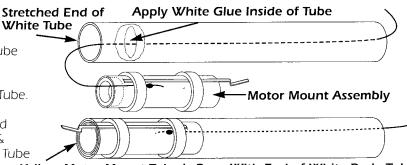
Yellow Motor Mount Tube is Even With End of White Body Tube
