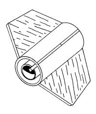
With white glue, glue the four fins to the template marks on the short tube. Wait for each fin to dry before applying the next.
