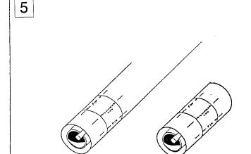
Wrap the fin template guide around both body tubes. Use a pencil and mark the fin and launch lug locations. Notice where the engine clips are in the drawing.
