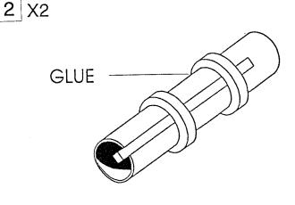
Apply white glue to the joints on all of the rings. Let this motor mount completely dry before going to the next step. It's very important not to rush this step!
