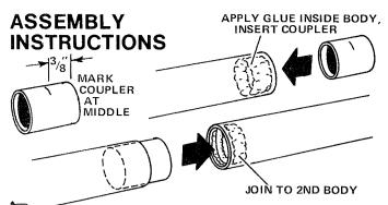
Assemble the main body. Mark the tube coupler (part I) at its middle. Smear glue around the inside of one end of a 12" body tube (part A). Insert the coupler into the glued body end so half of the coupler is in the tube. Let the glue set, then smear glue inside one end of the other 12" tube and slide glued end onto the coupler to join the tubes. Lay the assembly on a flat table top and roll gently to make sure the tubes are straight.
