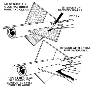
15 When all glue on the outside of the model is dry, prepare the balsa parts for painting. Apply at least two coats of sanding sealer to all wood surfaces. Let dry and sand lightly between coats. Do this until the tiny holes in the wood are filled and everything looks and feels smooth. After the sanding sealer
