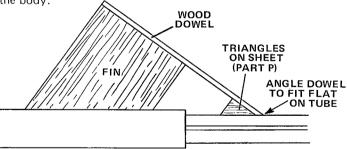
10 When glue applied in step 9 has completely hardened, cut lengths of wood dowel to fit along the top edge of each fin and extending down to the center body tube between trusses. Angle the end of each dowel to fit flush with the tube. When the glue has hardened, cut the small triangles out from balsa sheet (part P) and glue in the intersection of dowels and tube.
