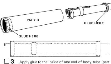
Apply glue to the inside of one end of body tube (part B) and to the adapter ring just forward of the engine holder. Slide body tube (part B) into place matching its ends with the adapter rings. Wipe away any exposed glue.
