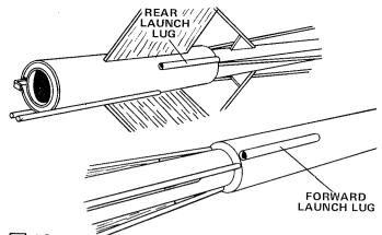
12 Glue the two launch lugs (part F) in position as shown. Make sure they are in line with one another and along side of one truss so launch rod does not rub on side of truss dowels.
