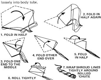
**T-13** Make as small a "package" of your "Solar Sail" as possible, see illustration above. "Sail" should slide easily in and out of body tube.
