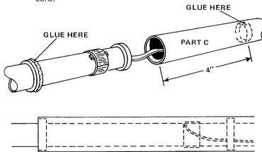
5 Glue body tube (part C) to the two forward adapter rings as shown. Use a small stick or dowel to apply glue to the inside of part C tube approximately 4" in from the rear end.
