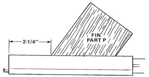
P) and gluing them in place 2-1/4" from the back edge of rear body tube. Make sure that each fin extends straight out from the body.
