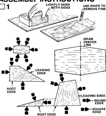
Fine-sand both sides of the balsa fin sheet (part A). Carefully remove the fins from the sheet using a sharp knife to free the corners and edges. Sand round the leading edges of the main wings and the leading edge of the vertical fin as shown. NOTE: The leading edge follows the direction of the grain. Place the horizontal fin on the above drawing. Draw the centerline as shown. Sand round all edges using the centerline as a guide to help prevent over-sanding one of the edges.
