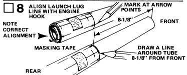
Carefully cut out the fin marking guide (part O) from back of the panel. Wrap the guide around the rear of the tube. Match the printed alignment marks, align the launch lug line with the engine hook, and tape the ends together. Mark all guide lines on the body tube. Using the front edge of the guide, draw a line around the body tube 8-1/8" from the front. Remove the guide.
