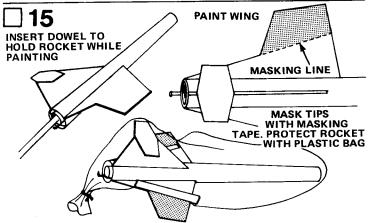
Use a wood dowel or similar object inserted in the rear of the rocket to hold it while painting. Spray the entire rocket with several light coats of gloss white spray paint. After this paint has thoroughly dried, mask off the wing tips on the top and bottom as shown. Paint the tips insignia blue. Carefully remove the masking tape and plastic bag from the model.
