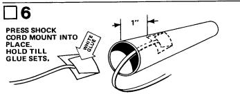
Smear glue over the entire backside of the shock cord mount. Hold the mount as shown and press it into place inside one end of the rocket body tube (part G). Make sure the front of the mount is at least 1" from the end of the tube. Hold the mount in place until the glue sets.
