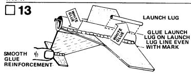
Glue the launch lug (part H) along the launch lug line so that the front of the lug is at the forward guide mark drawn in Step 8. Make sure the launch lug is aligned straight along the body tube. Apply a glue reinforcement to each fin joint. Holding the model level, apply a line of glue to both sides of each joint. Smooth out the glue with your finger. Keep the model level until the glue dries.
