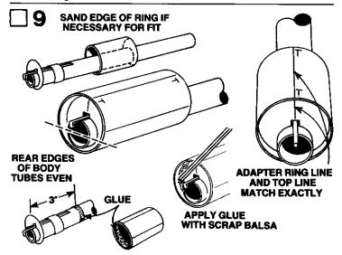
The glue should now be dry on the body tube/adapter ring joint (Step 6). Test-fit the body tube assemblies together as shown. If the rear adapter ring won't slide into the BT-55 tube, sand the edges of the ring
