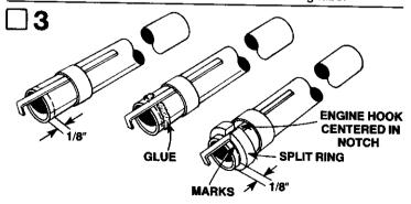
Mark the body tube 1/8" from the rear end. Place several marks around the tube so the centering ring may be accurately aligned. Apply glue around the tube above the marks, being careful not to get glue on the engine hook. Slide the split centering ring (part D) onto the tube and position ring with its rear edge on the marks. Hold ring in place until glue begins to set.
