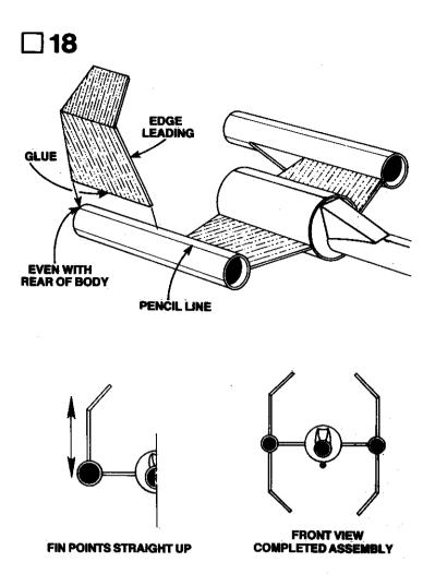
When attaching fin assemblies, keep in mind that the leading edges face forward and the angled portions of the fins point in toward the center of the body. Glue the fin assemblies in place one at a time, holding the fin in place pointing straight up or down until the glue sets. After the glue joints are completely dry, apply glue reinforcement fillets to all joints.
