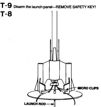
Slide the launch rod through rocket launch lug. Make sure the rocket slides freely on the launch rod. Clean the micro-clips and attach them to the igniter wires. Arrange the clips so they do not touch each other or the metal blast deflector. Attach clips as close to protective tape on igniter as possible. Check the micro-clips to make sure they cannot become entangled with the fins during launch.
