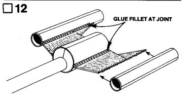
Apply a bead of glue to the outer edge of one wing. Attach one of the BT-20DJ tubes to it with a pencil line centered on the wing and the front edges of wing and tube even. Hold the assembly until the glue begins to set, then attach the second tube to the opposite wing. After the glue has dried, apply a bead of glue to both sides of the joints where the 3 body tubes join the wings. Smooth the glue into an even fillet with your finger.
