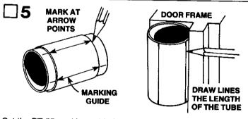
Cut the BT-55 marking guide from page 7 of the instructions. Locate the 2%" long BT-55J body tube (part F). Wrap the guide around the body and tape the ends together. Mark the tube at the arrow points. Remove guide and draw lines the entire length of the tube on the marks.
