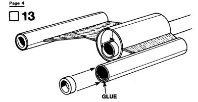
Glue the two AR-520 rings (part I) into the rear of the BT-20DJ tubes.
