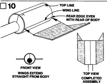
Test fit a wing to the body as shown. Make sure you have the wing positioned just as shown in the drawing. Apply glue to the inside edge of the wing and attach to the body, centered on the wing line. Make sure the wing points straight out from the body. Support with the wing pointing straight up until the glue dries. Attach the other wing to the opposite side of the body in the same manner.
