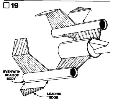
Glue the two winglets to the outside of the BT-20DJ tubes. Apply glue fillets along joints.
