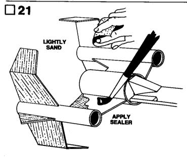
Seal all balsa parts with sanding sealer. Allow the sealer to dry and lightly sand the parts. Seal and sand again. A third or even fourth application may be necessary to achieve a smooth, grain-free surface.
