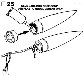
Apply plastic model cement (tube type or liquid) around the inside of the end of the nose cone (part R). Socket the base (part S) in place. NOTE: <u>DO NOT USE WHITE GLUE FOR THIS</u>. Allow cement to dry. Tie the end of the shock cord to the nose cone, tie a triple knot. Roll up the chute and shroud lines and push them, along with the shock cord, down into the body tube. Socket the nose cone into place.
