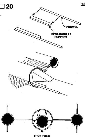
Cut the 6" dowel (part M) into two 3" lengths. Glue a rectangular support to each dowel. Glue the assemblies to the body on the guide lines on either side of the cockpit.
