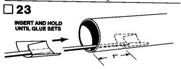
The shock cord is glued into the front of the body tube 1" from the end. This allows clearance at the front of the tube for the nose cone to socket into place. Use a stick to deposit a generous dab of glue inside the body tube, 1" from the end. Slide the shock cord mount into the tube and press into the glue. To insure a good bond, use the stick or your finger to smear a film of glue over the mount and the surrounding area in the body tube.
