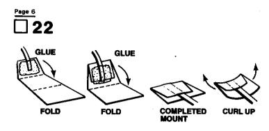
Cut out the shock cord mount from page 7 of the instructions. Fold on dotted lines, then unfold and apply glue to Sec. 1. Lay the end of the shock cord (part N) in the glue. Fold over and apply glue to the back of Sec. 1 and the exposed part of Sec. 2. Fold again to complete mount. Curl the edges of the mount up so it will match the contour of the body tube and hold with your fingers until the glue sets.
