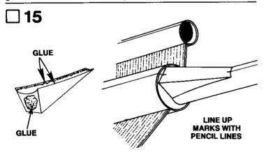
Proceed with this step only after the glue on the cockpit is completely dry. Apply a bead of glue to the inside edge of each side and to the back of the cockpit. Set the cockpit in place as shown (note how marks on cockpit line up with pencil lines on body). Hold the sides of the cockpit against the body until the glue sets. Use a small stick or toothpick to apply a thin bead of glue all around the body-cockpit joints. Run your little finger along the joints to smooth out and remove excess glue.
