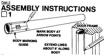
Cut the BT-20 marking guide from page 7 of these instructions. Wrap the guide around the 12" long BT-20L body tube (part A) and tape the ends together. Mark the body tube at each of arrow points. Remove the guide and lay it aside (it will be used again later). Using a door frame as a guide, draw lines connecting the marks. Extend the lines about 6" from the end of the tube.
