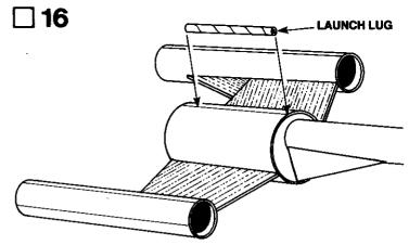
Glue the launch lug (part K) to the bottom of the BT-55 body, centered on the bottom pencil line, with the front of the body and lug even. Apply a light bead of glue to both sides of the launch lug to strengthen the joint.
