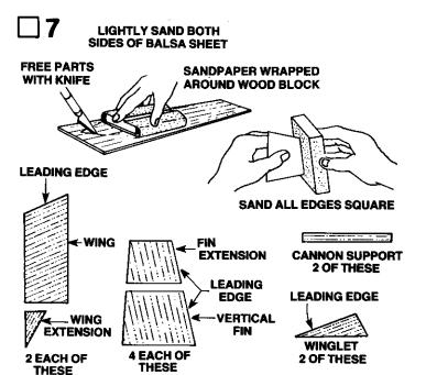
Lightly sand both sides of the balsa die-cut sheet (part G). Carefully free the parts from the sheet using a hobby knife. Lightly sand the edges of all parts, making sure the edges remain square. Lay out and identify the parts as shown above. Note that the balsa grain line runs parallel to the leading edges of the parts.
