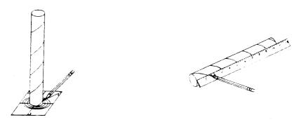
\_\_\_\_1. Using the fin alignment guide mark lines on the long body tube for fin alignment as shown.
