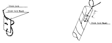
3. Install the shock cord mount as shown. Spread a heavy layer of glue over the shock cord mount on the side opposite the shock cord knot. Curve the shock cord mount and insert into the nose cone end of the body tube. Press firmly in place. Be sure the mount is at least 1" inside or the nose cone will not go in the body tube. The drawing shows the proper positon inside the body tube.
