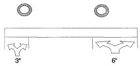
3) Glue the inner tube assembly into the body tube. The inner and outer tubes should be flush top and bottom.
