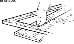
6 Put a layer of glue on the root of each fin where it will be joined to the body tube. Do not glue to the body tube at this time. Set each fin aside to dry. You are making a "double glue" joint that will later be very strong. This is the first step in making a double glue joint.
