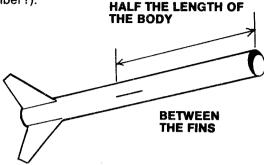
13 Glue the launch lug to the body making sure that it is lined up fore-and-aft and is NOT in line with any fin.
