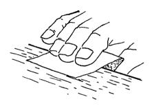
Put a coat of "sanding sealer" on the balsa parts and body tube. This special paint is available at hobby shops. Its purpose is to seal the balsa wood to prevent paint from soaking into it. It will give you a lighter model. After the sanding sealer has dried, do not sand it.
