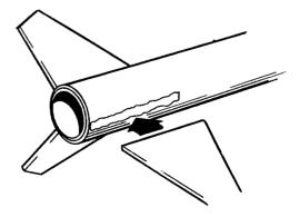
12 Measure for the location of the launch lug on the body tube. It must NOT be in line with a fin, or the launch rod will not be able to go through it. It should be located out of line with the fins and half-way along the body tube. Measure its location. Mark the location with a pencil. Apply a thin layer of glue to the body and to the lug (make a double glue joint, remember?).
