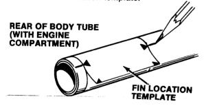
8 Using the edge of a drawer or other V-shaped piece as shown in the drawing, draw a line with the pencil up the tube from each place you have marked a fin location with the fin template. These lines should be drawn straight up the tube. You will use them later to make sure that the fins are glued on straight and in the proper location.
