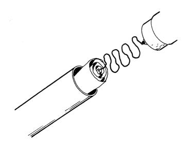
Install the nose cone on the front of the body tube. If it is too tight, sand it down until it slides on and off easily. If it is too loose, build up the shoulder with one or two layers of tape. Make sure that shroud lines, shock cord, etc.arenot jammed between the nose cone shoulder and the front of the body tube.
