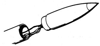
Install the electric igniter into the engine nozzle according to the instructions that come with each MINIJET engine pack. Most ignition failures occur because the modeller does not install the igniter AS FAR AS IT WILL GO into the nozzle and because he does not press the tape down onto the nozzle AS TIGHTLY AS POSSIBLE. Experienced model rocketeers always check these little points and rarely suffer from mis-fires.
