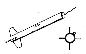
14 Tie the free end of the shock cord to the screw eye in the base of the nose. Use two or three knots. Make them tight.
