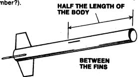
13 Glue the launch lug to the body making sure that it is lined up fore-and-aft and is NOT in line with any fin.
