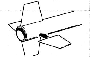
Measure for the location of the launch lug on the body tube. It must NOT be in line with a fin, or the launch rod will not be able to go through it. It should be located out of line with the fins and half-way along the body tube. Measure its location. Mark the location with a pencit. Apply a thin layer of glue to the body and to the lug (make a double glue joint, remember?).
