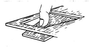
6 Put a layer of glue on the root of each fin where it will be joined to the body tube. Do not glue to the body tube at this time. Set each fin aside to dry. You are making a "double glue" joint that will later be very strong. This is the first step in making a double glue joint.
