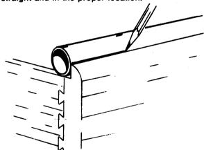
9 Put a thin layer of glue on the body tube where you will later glue the fins. Let this layer of glue dry. This is the second step in making a strong double glue joint.
