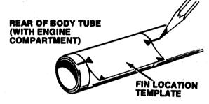
B Using the edge of a drawer or other V-shaped piece as shown in the drawing, draw a line with the pencil up the tube from each place you have marked a fin location with the fin template. These lines should be drawn straight up the tube. You will use them later to make sure that the fins are glued on straight and in the proper location.
