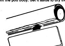
Glue the launch lug to the left hand side of the pylon where it joins the pod body. Make sure it is lined up fore-and-aft.
