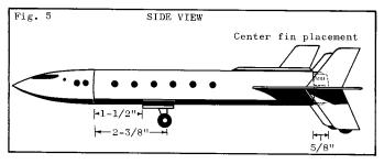
7. Apply glue to the root edges of the upper tip fins and position them on the topside of the main fins on the location marks. Glue the center fininto place on  $\underline{top}$  of the launching lug, positioning it as shown in Fig. 3 and Fig. 5. Apply glue to the root edges of the lower tip fins and place them on the lower side of the main fin directly under the upper tip fins as shown in Fig. 3. Allow to dry.
