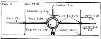
5. Mark the body tube for the positions of the main fins, launching lug and bottom centerline. Draw guide lines from these marks so that all lines parallel the tube centerline. Smear a liberal amount of glue 1-1/2" up into the rear end of the body tube. Push the engine holder assembly into place until the mark (made as in Fig. 2) on this assembly is even with the rear of the body tube. Glue the launching lug and the main fins in their positions and stand the assembly aside to dry.
