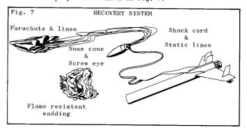
10. Prepare the COMMUTER for flight in the usual way. Insert wadding, parachute, shroud lines and shock cord into the forward end of the body tube. Gather the static lines so they meet at the forward edge of the body tube on top, and push the nose cone into place. The COMMUTER flies well with any Series I single stage engine.
