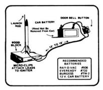
LAUNCH SYSTEMS: An Estes electrical launch system is recommended for all model rocket launching. Some rocketeers, however, prefer to design and build their own launching systems. A simple homemade launching system is illustrated.
