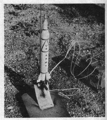
Above: The bird is all set and ready to launch. A board, some sheet aluminum, and a piece of 1/6" plano wire suffice for a pad. The motor is the popular "Rock-A-Chute" unit which can be bought at many hobby shops. Ignition is obtained through the use of a 6-volt battery supply and a remote firing switch.
