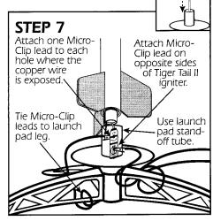
IMPORTANT: To avoid potential short circuit and/or misfire DO NOT clamp Micro-Clips too tightly to the Tiger Tail II igniter.
