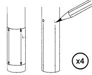
pairs of points with straight lines running at least 2" from the end of the body. Mark one of the lines L and one R as
