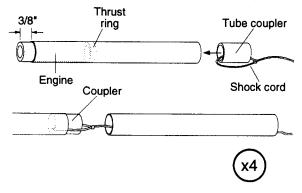
down the outside of the coupler. Glue the second body tube to the coupler, making sure the two sections are straight. Repeat to make four MIRV bodies.
