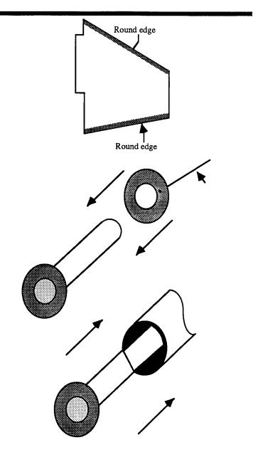
8) Epoxy the fins into the fin slots in the body tube. Make sure they are straight with the body tube. For maximum strength give the fins a good fillet coat of epoxy.
