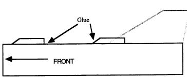
9) Epoxy the bulkhead into one end of the tube coupler. Epoxy the screw eye into the bulkhead. Epoxy the tube coupler halfway into the payload tube.
